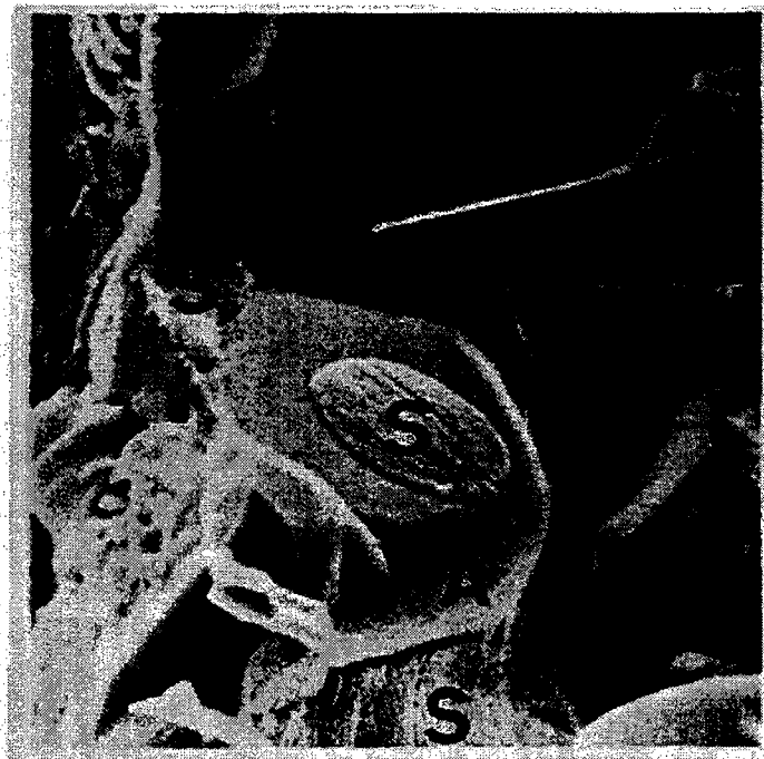
Plate 21 Idiomorphic alite (A) embedded in sulfate-rich matrix (S). 2000 x
